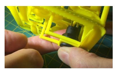
This photo shows a closeup of the connectors after they have been attached to the bottom of the pushbutton.
