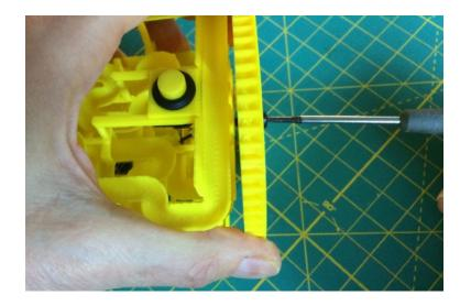
Tighten the axle screw all the way, then back it off about a quarter of a turn. You want a small gap between the maze and the lifting gear, so that the gear will turn freely, but you don't want it so loose that it wobbles.
