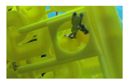
Remove the black plastic nut from the Pushbutton and hold it below the pushbutton mounting hole on the top of the maze. Route the Motor Assembly connectors through this nut. Make sure that the "ratchet" side of the nut is pointing towards the Pushbutton mounting hole in the Maze. It may help to hold the wires with tweezers.
