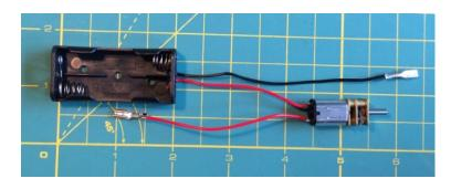
Temporarily install two AAA batteries into the battery holder and hold the on/off pushbutton terminals together. Make sure the motor is rotating in the clockwise direction when looking at it's axle, as shown in this picture.
