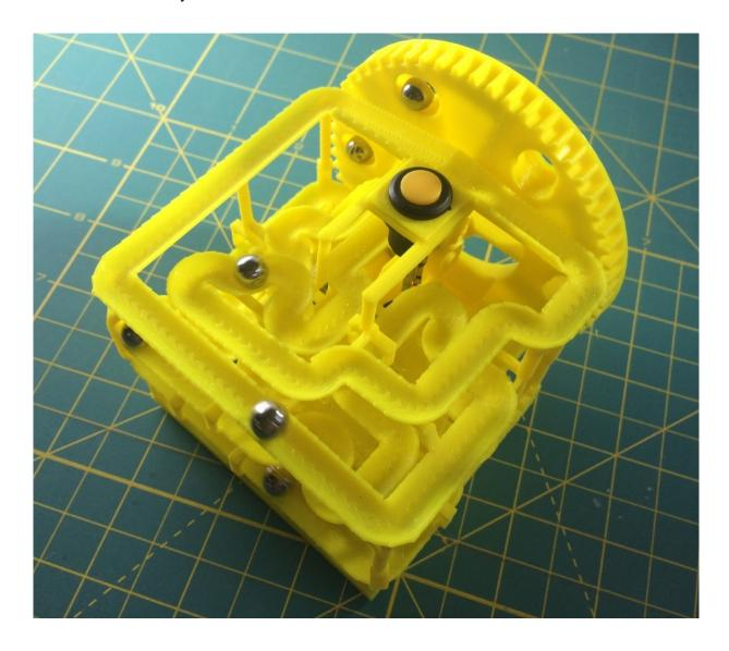
If the balls stop rolling after a while, find where they are getting stuck and clean out whatever is obstructing the paths. If the balls are falling off the track, there could be stray plastic obstructing them, or you're table may not be level.
