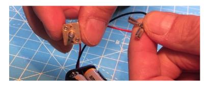
Insert the motor through the gap between the motor mount and the battery compartment locations as shown here.
