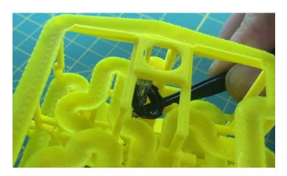
Push the connectors up through the round mounting hole and attach them to the Pushbutton.
