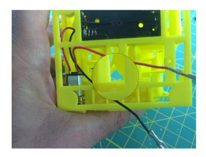
Viewed from above it looks like this. (This picture is looking through the pushbutton mounting hole on the top of the model down towards the triangular passage the connectors are routed up through).
