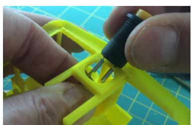
Insert the pushbutton into the top of the mounting hole and finger-tighten the nut. Note that the model is being held upside down in this photo.
