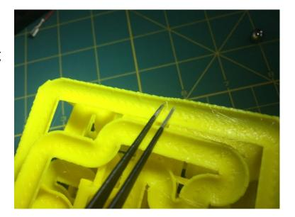
Be sure to inspect the Lifting Gear as well. The six ball chambers in the Lifting Gear should all look the same, although rotated differently with respect to the gear. If you see excess plastic in the holes clear it away with tweezers or a knife.
