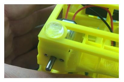
Attach the Motor Gear. Notice that the tapered side points outwards from the Maze.
