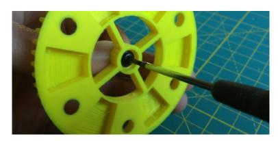
Make sure the lifting gear spins freely. The axle shouldn't fit too tightly, but you also don't want it too loose. It may be necessary to spin it with your finger a few times to get it to loosen up.
