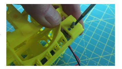
Route the pushbutton connectors between the two bottom tracks and up through the small somewhat triangular opening (magnified in this picture).
