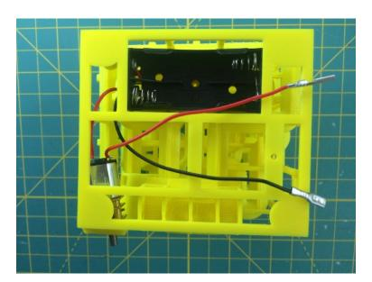
Attach the battery box using the 2mm diameter tapered screw.
