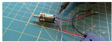
Hold the two pushbutton connectors together and make sure the motor is turning clockwise.
