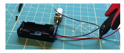
Trim the black wire to 4.0 inches, and strip about 1/4 inch of insulation from its end. You can discard the unused portion of black wire.
