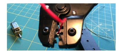
Or, use a pair of pliers to close the connectors wings around the wires.
