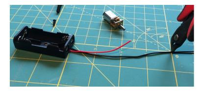
Attach the black wire from the battery box to one of the pushbutton crimp connectors, and the extra piece of red wire to the other connector. (If you don't have a crimping tool it is a good idea to solder the wires to the connectors).
